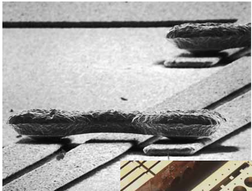
Airbridges is an ideal technique for implementing PCB crossovers with excellent high-frequency characteristics. The above photo has been taken with a scanning electron microscope and shows such an airbridge which is only 0.05 mm long.
